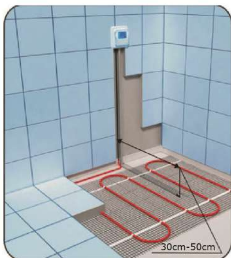
Diagram of temperature sensor placement in corrugated pipe
